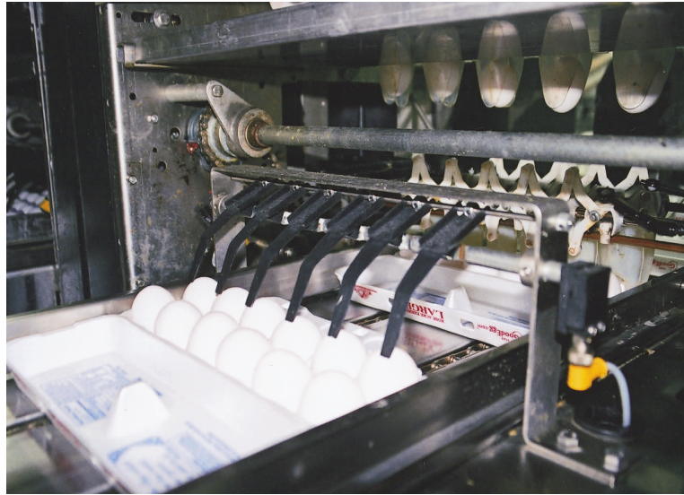
Each packing line provides six lanes into which the eggs are fired. When six eggs are present, the machine indexes them forward and lowers them, small-side-down, into open cartons below, left. Filled cartons move underneath a missing egg detector, above, that will stop the process if an egg is missing.
