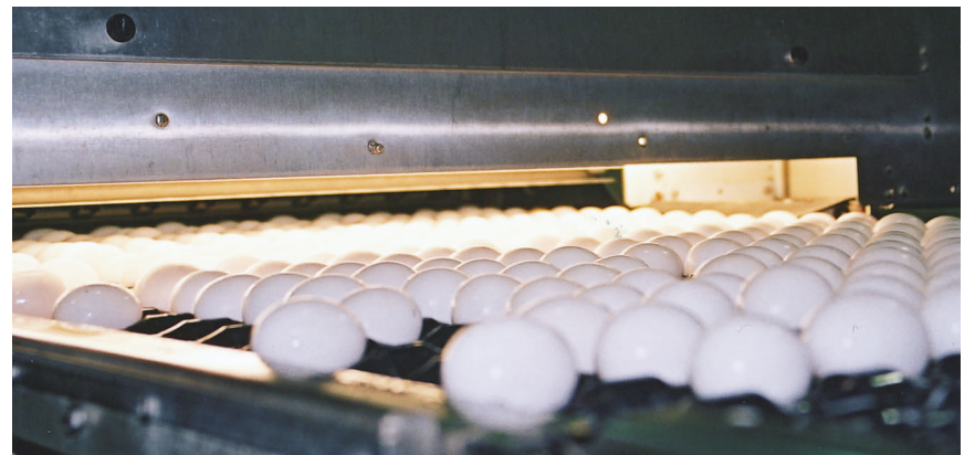
Eggs move through a blood-detection system, above, that shines a light through the eggs to see if there are any blood spots within. Egg cartons are coded by a four-line ink-jet printer, at top of page, left, with the Julian date, plant number and sell-by date.
