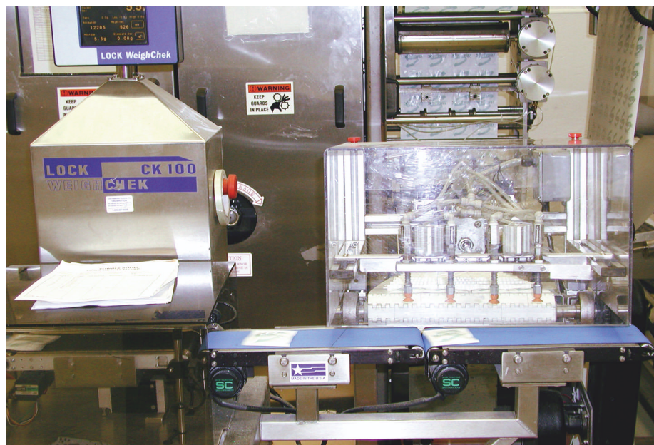
Checkweighers were added to three lines, the most recent of which is linked with a custom, side-transfer system for speedy weighing of solid-dose products and powders. The transfer unit both automates the transfer process and effectively spaces the containers.
