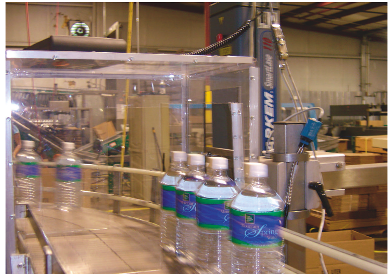
Bundles of bottles are depalletized as water from the springs is pumped to the filling station from holding tanks. After filling and capping, the bottles are labeled with paper labels and proceed on a conveyor to the laser coder, above and top. While line speeds (about 250 bpm) aren't necessarily higher, Natural Springs says line efficiencies and coder reliability have greatly improved.
