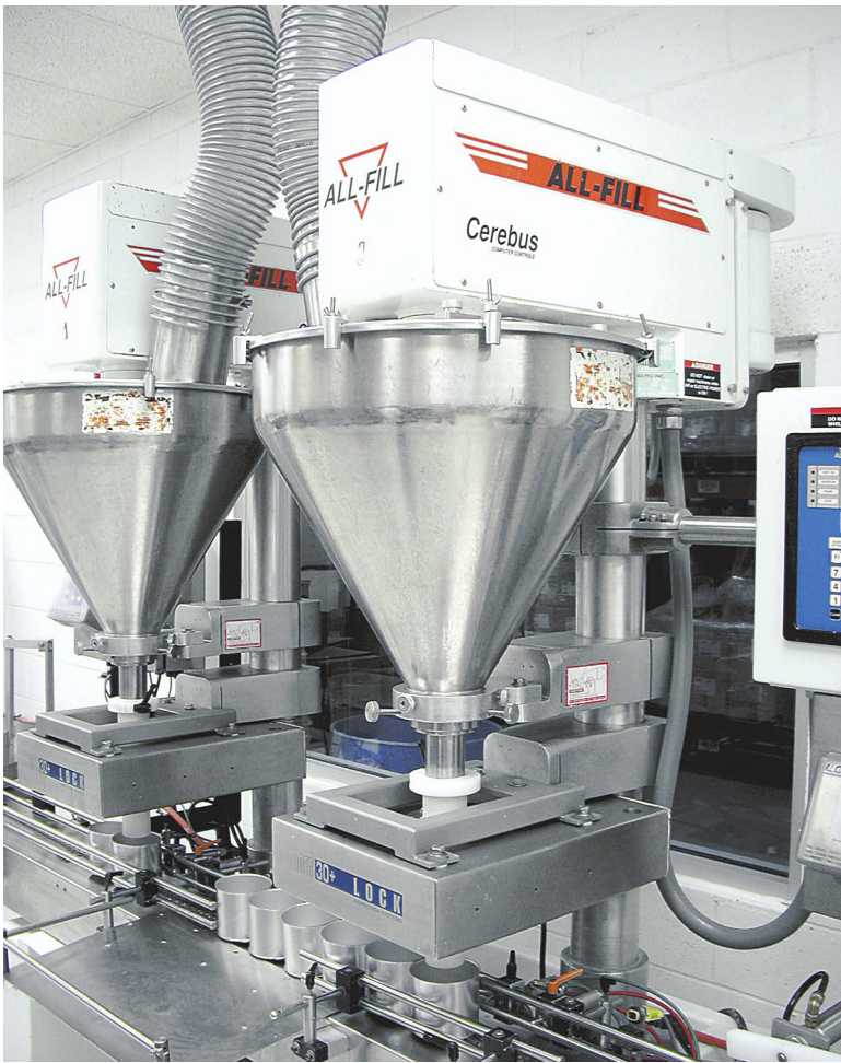
Examples of the many thousands of products and packages Garden State fills appear below. Compact metal detectors were installed on auger filler lines, left, to fit into tight spaces.
