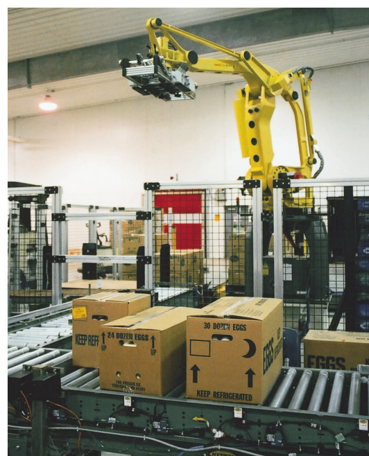
A portion of the cases are palletized through the use of a four-axis, electric, servo-driven robot that can handle four different case sizes at one time.
