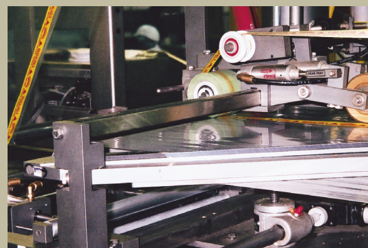
Standalone unit applies tape to film as it enters the vf/f/s machine, top. A wheel perforates the film so the top can be torn off of the bag by the consumer.
