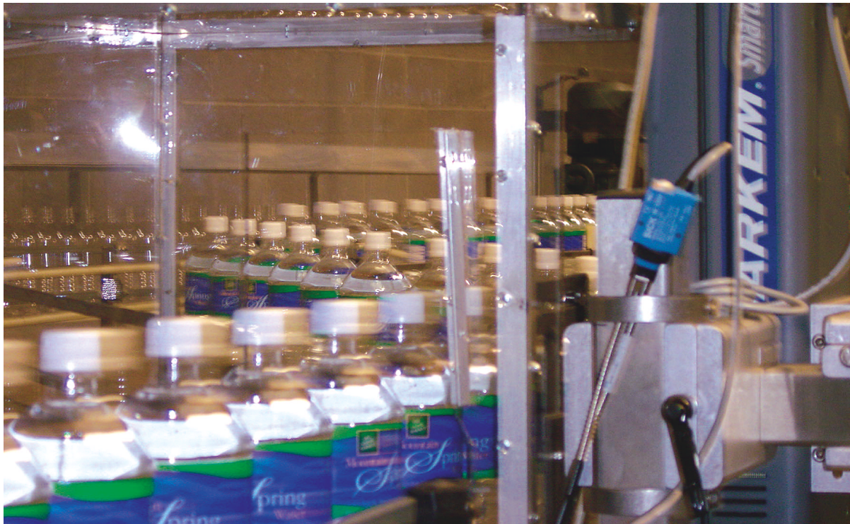
Filled, capped, labeled bottles of Natural Springs water convey in single file to the laser-coding station where they receive a open date code on the side. The line outputs about 250 containers/min.
