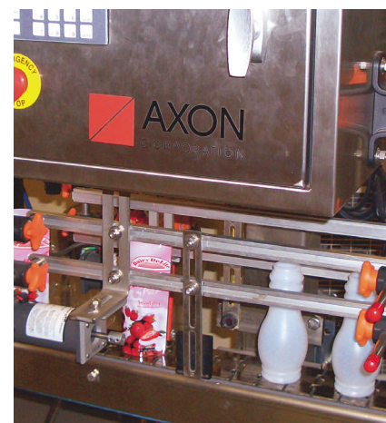
Above and below, Noga's dairy bottles enter the sleeve applicator/shrink tunnel combination system, which operates at speeds up to 150 containers/min with labels up to 80 mm dia.
