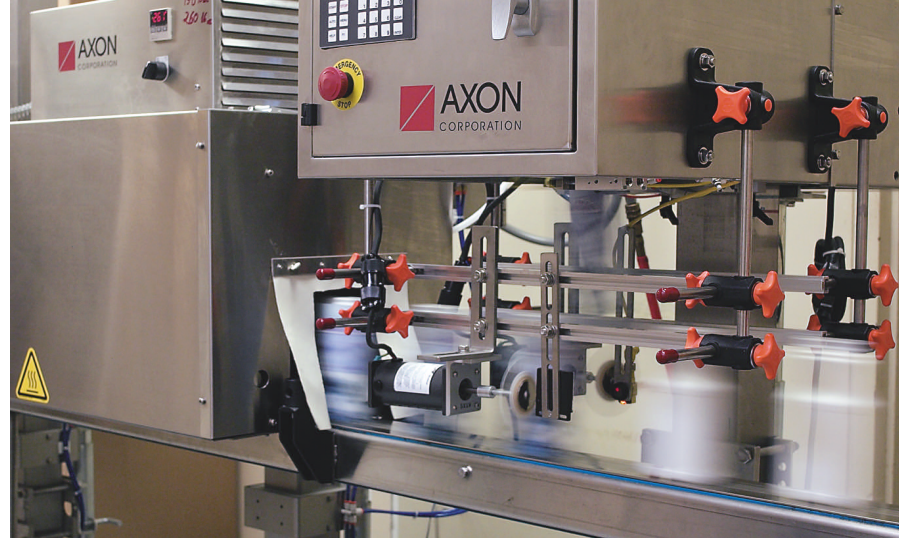
Above and below, Noga's dairy bottles enter the sleeve applicator/shrink tunnel combination system, which operates at speeds up to 150 containers/min with labels up to 80 mm dia.
