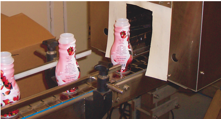
Noga Dairy's new teardrop-shaped bottles enter the single-head sleeve applicator, top, which applies a sleeve label over each container after it cuts the sleeve from rollstock. Next, the bottles move into the shrink tunnel, above, which snugly heat-shrinks the labels onto the shapely bottles for a tight fit.
