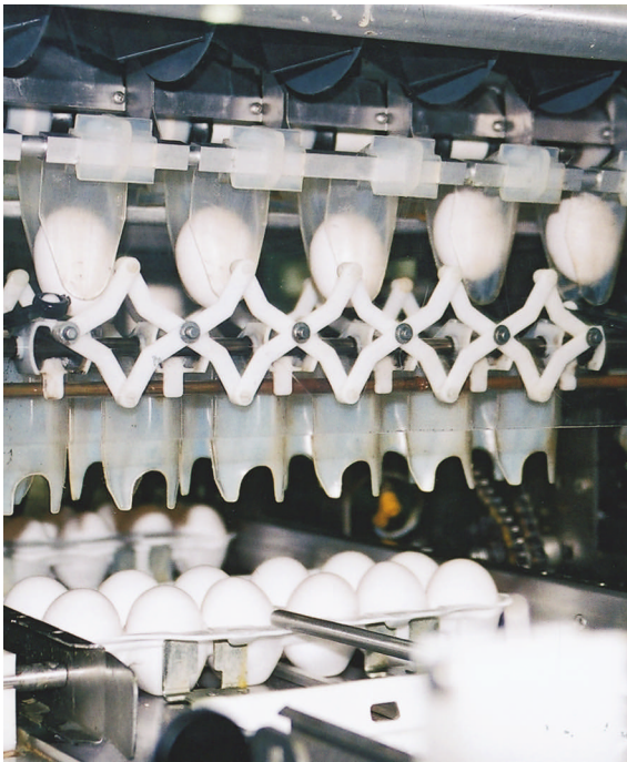
Each packing line provides six lanes into which the eggs are fired. When six eggs are present, the machine indexes them forward and lowers them, small-side-down, into open cartons below, left. Filled cartons move underneath a missing egg detector, above, that will stop the process if an egg is missing.
